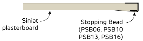
FIGURE 104 Finishing Detail - Stopping Bead Section
