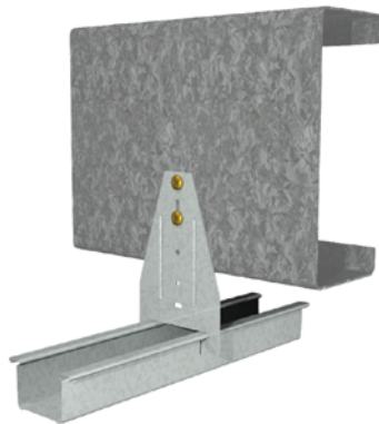
FIGURE 15 A Clip and Furring Channel Perspective and Sections
